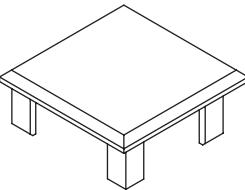
A small, square, flat metal cap with a thin profile, used to cover the top of a post.                                                |
