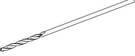
A long, thin, tapered metal bit with a spiral edge, used for drilling holes in wood.                                              |
