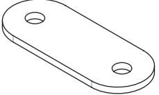
A small, oval-shaped metal clip with two circular holes, used to join two pieces of wood together.                               |
