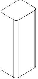
A rectangular, thin metal spacer used to maintain a consistent gap between the top of a post and the bottom of a horizontal board. |
